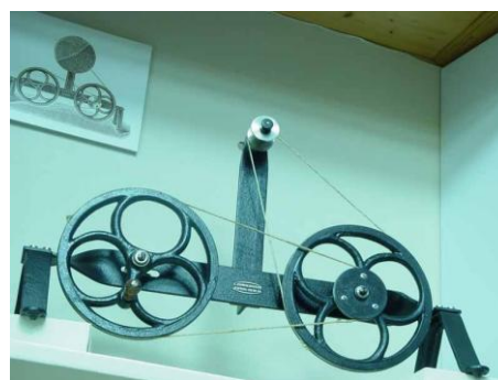
Manual colour rotator. Used for rotation of the Maxwell disk, through which the ability to recognize the density and brilliance of colours can be identified.
